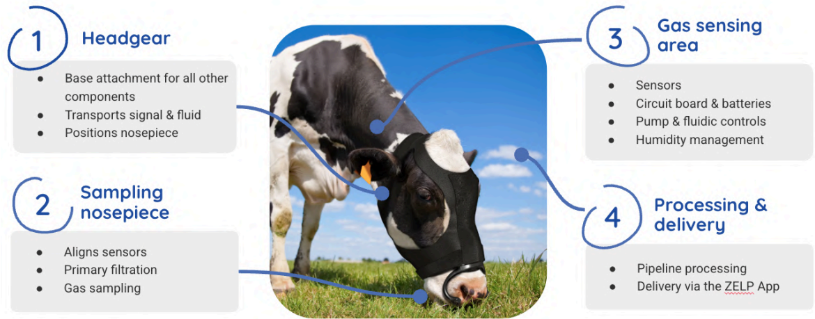
Figure 3. Full depiction of the Sense device and the usages of each component.
